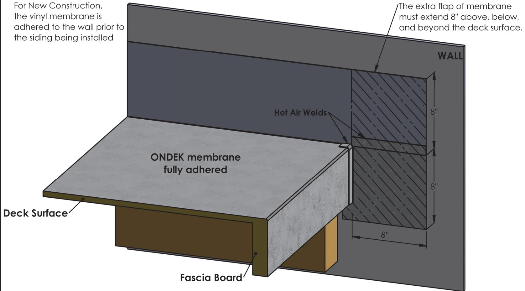
The flap is left loose so that the Sider can tuck it under the wall paper when it is applied.
